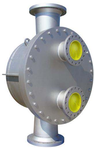
The SPS plate heat exchanger uses laser welded cassettes, which are made up of two round plates welded together using modern laser welding machines.
